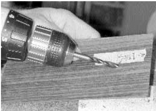
28. Hold the overlay in one hand and elongate the hole by slowly tilting the overlay against the running drill bit.
