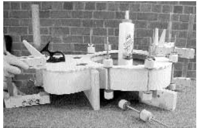
6. Start clamping in the waist area, for several inches to either side of the waist clamp, using spool clamps to gently hold the top in place.
