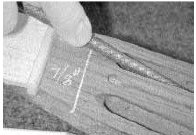
29. Carve and file ramps at the nut end of each channel so the strings don't rub wood on their way to the tuning posts.
