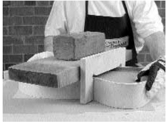
5. Try using a weighted board placed across the top side of the rim for uniform downward pressure.
