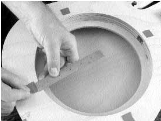
42. Measure 5/16" out from the edge of the soundwell rim on the centerline, and at right angles to it, and place a piece of masking tape at each point.
