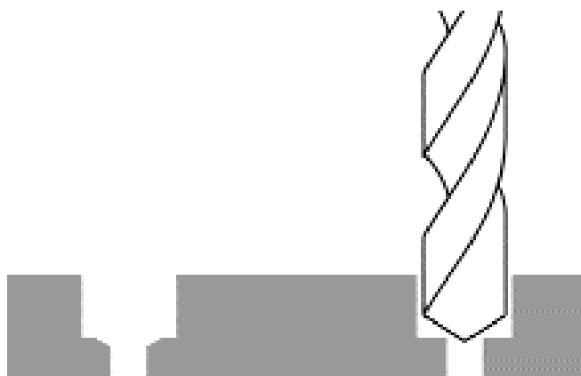
14. Create chamfers within the four 1/4" holes using a 7/32" twist drill.
