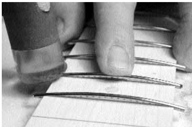
15. Keep the wire from tipping and prying up a chunk of wood as you tap the two ends into the fret slot with a hammer.
