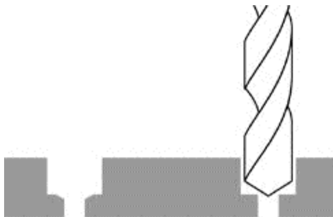
26. Create chamfers within the four 1/4" holes using a 7/32" twist drill.
