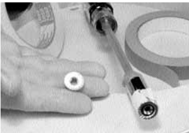
39. We made a long-handled nut driver from a deep-well, square-drive 7/16" socket, and a #3 Phillips screwdriver that fit the 1/4" drive perfectly.
