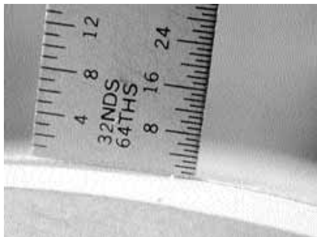
18. The router bit will cut slightly deeper than the actual thickness of the binding \frac{1}{32} perhaps by as much .007".
