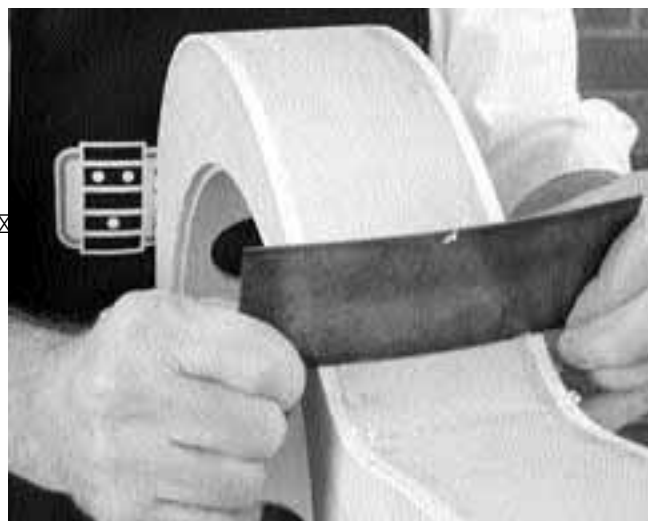
19. Scrape the wood to meet the binding all around the sides.
