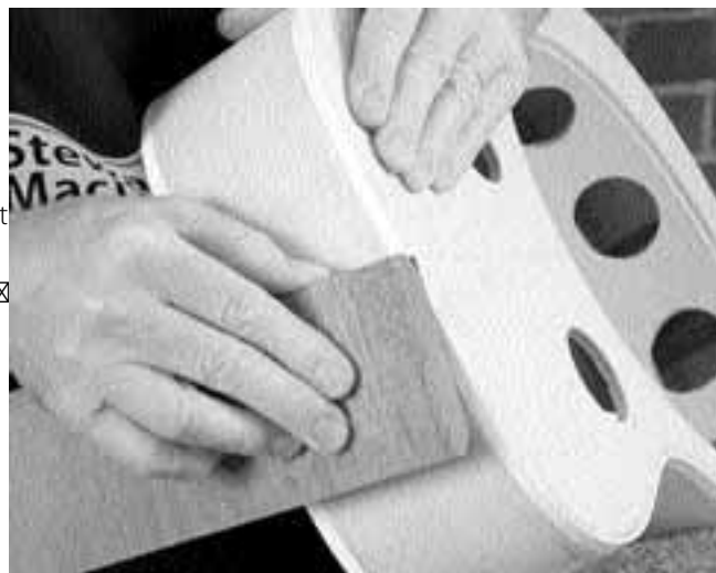
20. Use a flat block and 80- or 100-grit Fre-Cut sandpaper to flatten only the area of the sides at the neck block where it mates with the flat cheeks of the neck.
