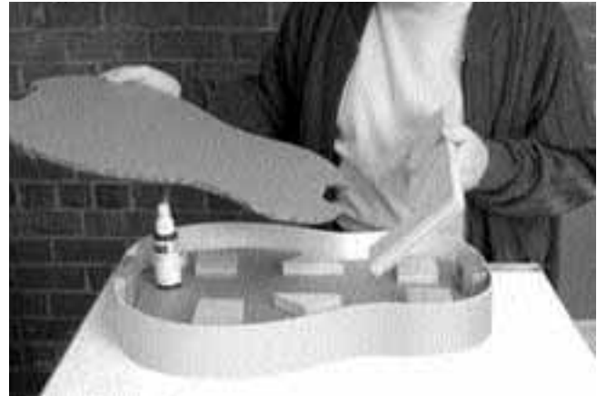
2. The two cardboard forms are fastened together with blocks of wood between them, creating a three-dimensional form for supporting the guitar sides.
