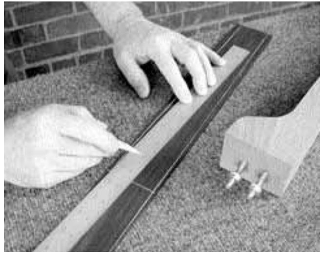
24. Draw the profile of the neck xxx taper onto the fingerboard using a white pencil.
