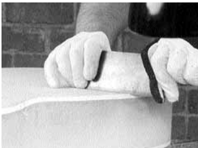
17. Use a sharp scraper to flush the binding to the wood.
