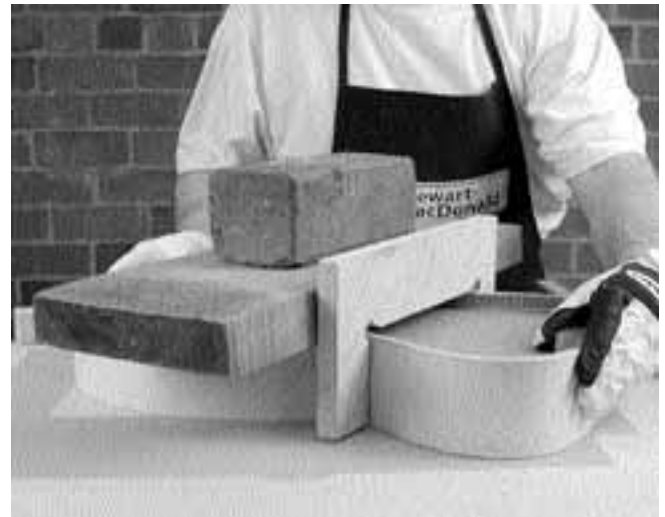
5. Try using a weighted board placed across the top side of the rim for uniform downward pressure.
